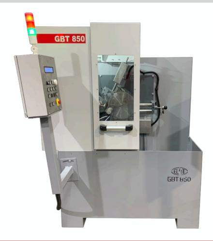
The ELITE model GBT 850 DUO is our CNC grinding machine for the flanks for circular saws with tungsten carbide teeth.
