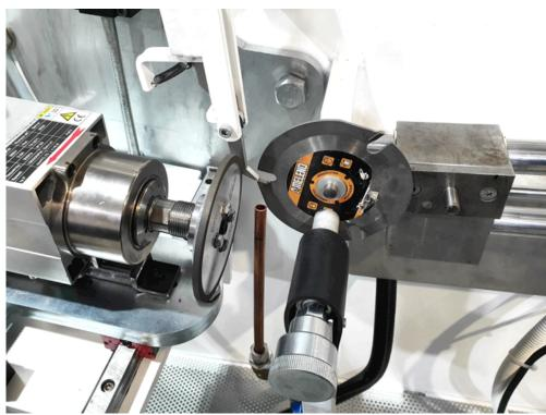
Saw diameter from 100 mm. For grinding the flanks of scoring discs or portable machines. Allows the indexing of any type of tooth pitch.
