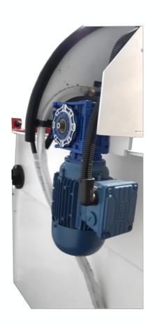
Grinding carriage translated by a poweful motor with worm reducer
