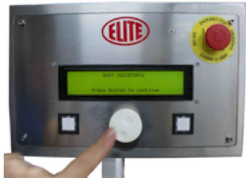
Control panel to adjust the direction of wheel rotation and speed depending on the diameter, as well as the different programs available as an option.
