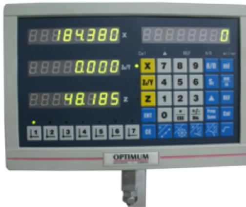
Control panel with digital scale position indicator. Up to 3 axis: X, Y, Z available as an option.
