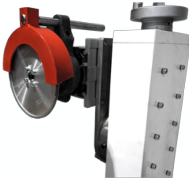
Detail of grinding wheel holder with protection for grinding wheels up to  $\varnothing 150$  mm. The grinding wheel head can be rotated  $360^\circ$  with respect to its vertical axis and  $90^\circ$  with respect to the horizontal axis.
